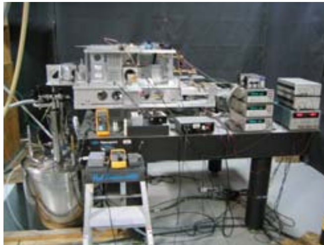
Figure 1. A 'quasi-optical' electron paramagnetic resonance (EPR) spectrometer.
