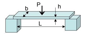
Strength – elastic flexural formula shows the maximum stress occurs at the extreme fibers of the beam at midspan
