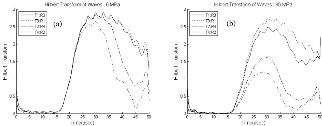
**FIGURE 6.** Hilbert transform of S0 mode signals; vertical wave propagation (a) unloaded, (b) 86 MPa far field static stress in vertical direction.
