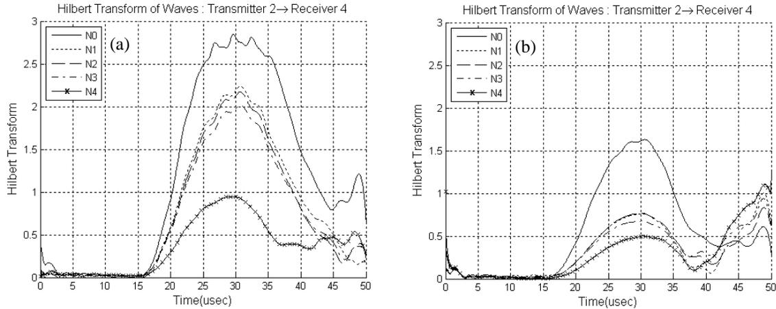
FIGURE 8. Fatigue crack effect on received signal (a) unloaded, (b) 86 MPa far field stress.
