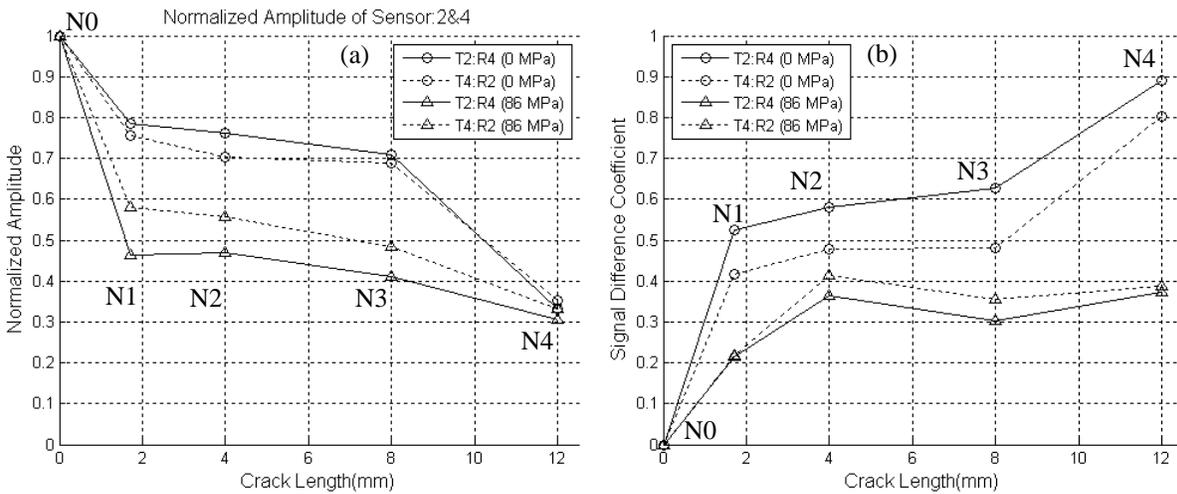
FIGURE 9. Effect of fatigue crack growth on (a) normalized amplitude of S0 mode, (b) signal difference coefficient for  $20 < t < 40$  us.
