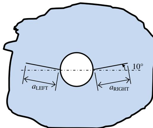
**FIGURE 4.** Schematic of fatigue crack growth from 12.7 mm diameter hole.
