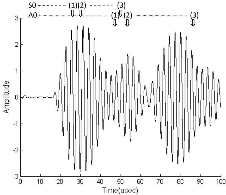
**FIGURE 5.** Initial A-scan (no load, no crack) for transducer path T2-R4 showing predicted arrival times for S0 and A0 wave modes.
