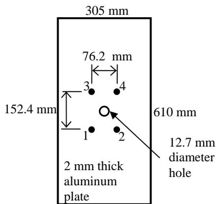
**FIGURE 3.** Transducer layout for single-hole plate sample.
