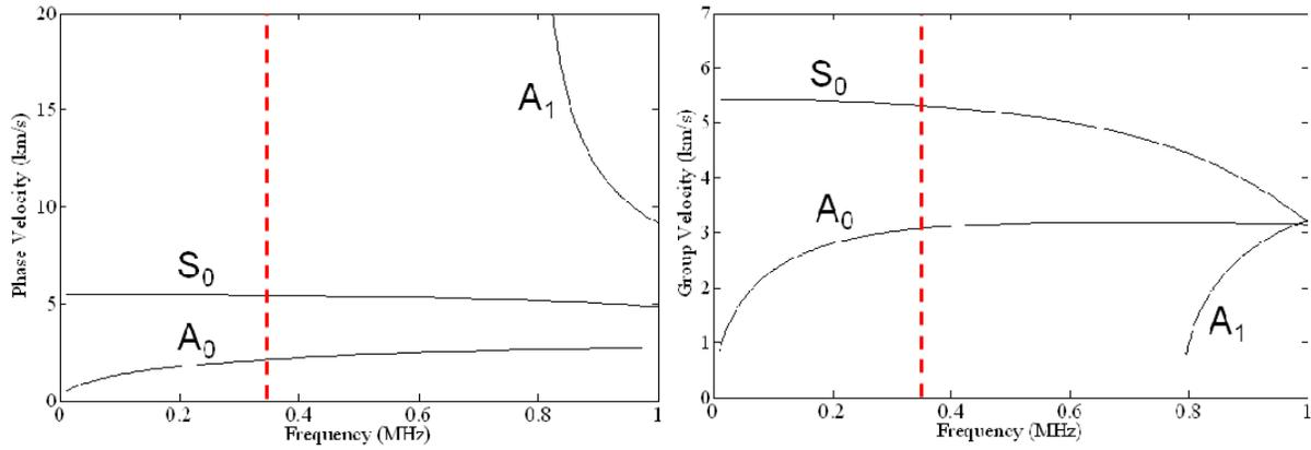
**FIGURE 1.** Phase and group velocity dispersion curves for a 2 mm thick aluminum plate with the 350 kHz central frequency of the transducers shown.
