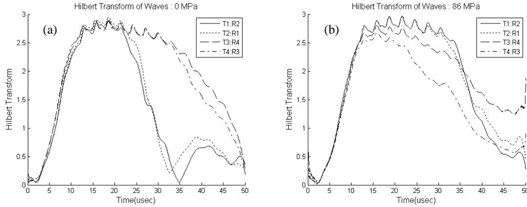
**FIGURE 7.** Hilbert transform of S0 mode signals; horizontal wave propagation (a) unloaded, (b) 86 MPa far field stress in vertical direction.
