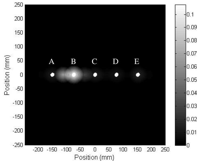
**FIGURE 2.** Tomogram showing location of 6 mm long EDM slot cut from left side of second 12.7 mm diameter hole.
