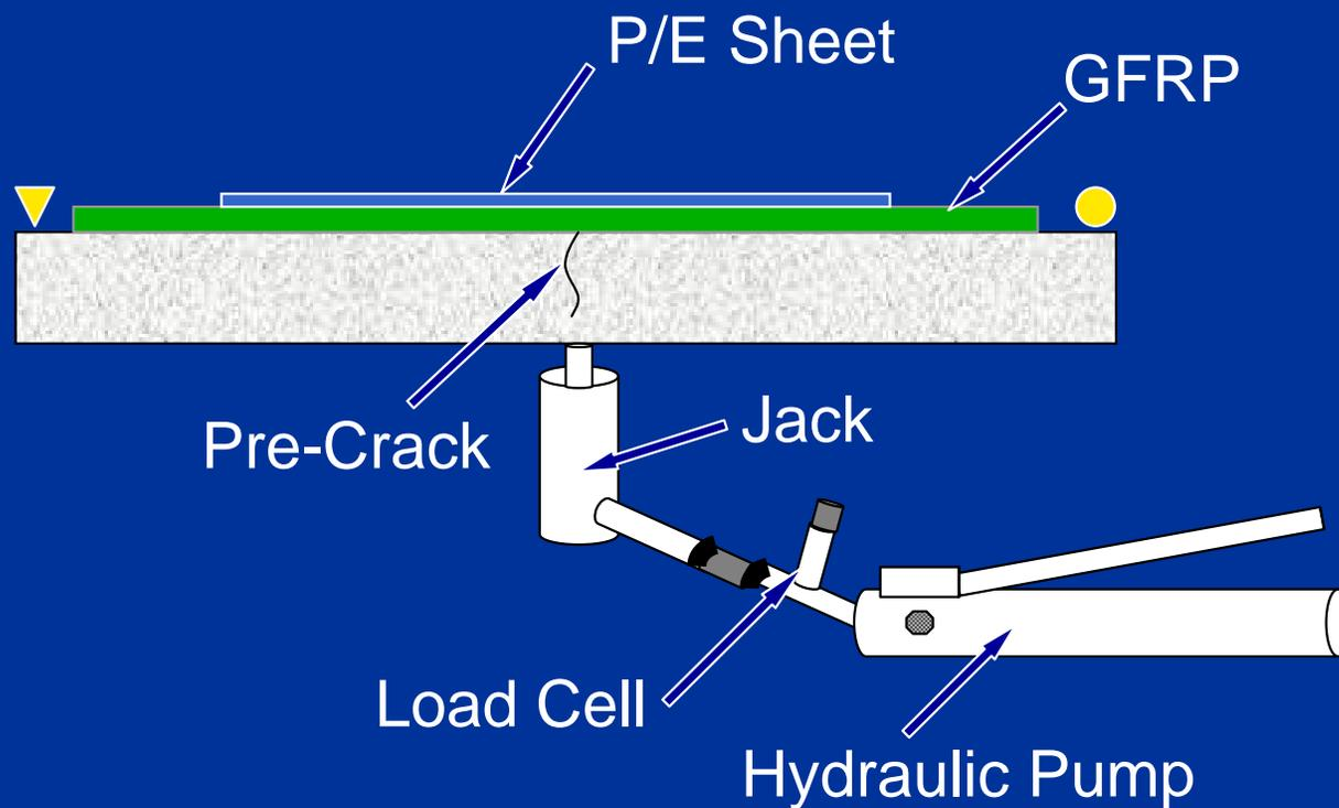
Full-field strains in GFRP sheet measured with photoelastic (PE) coating applied to tensile surface
