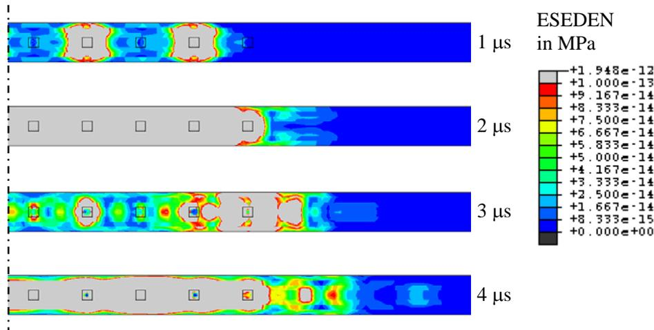
**Figure 6: Finite element simulation of generation of waves from embedded piezoelectric fibers in a CFRP laminate.**
