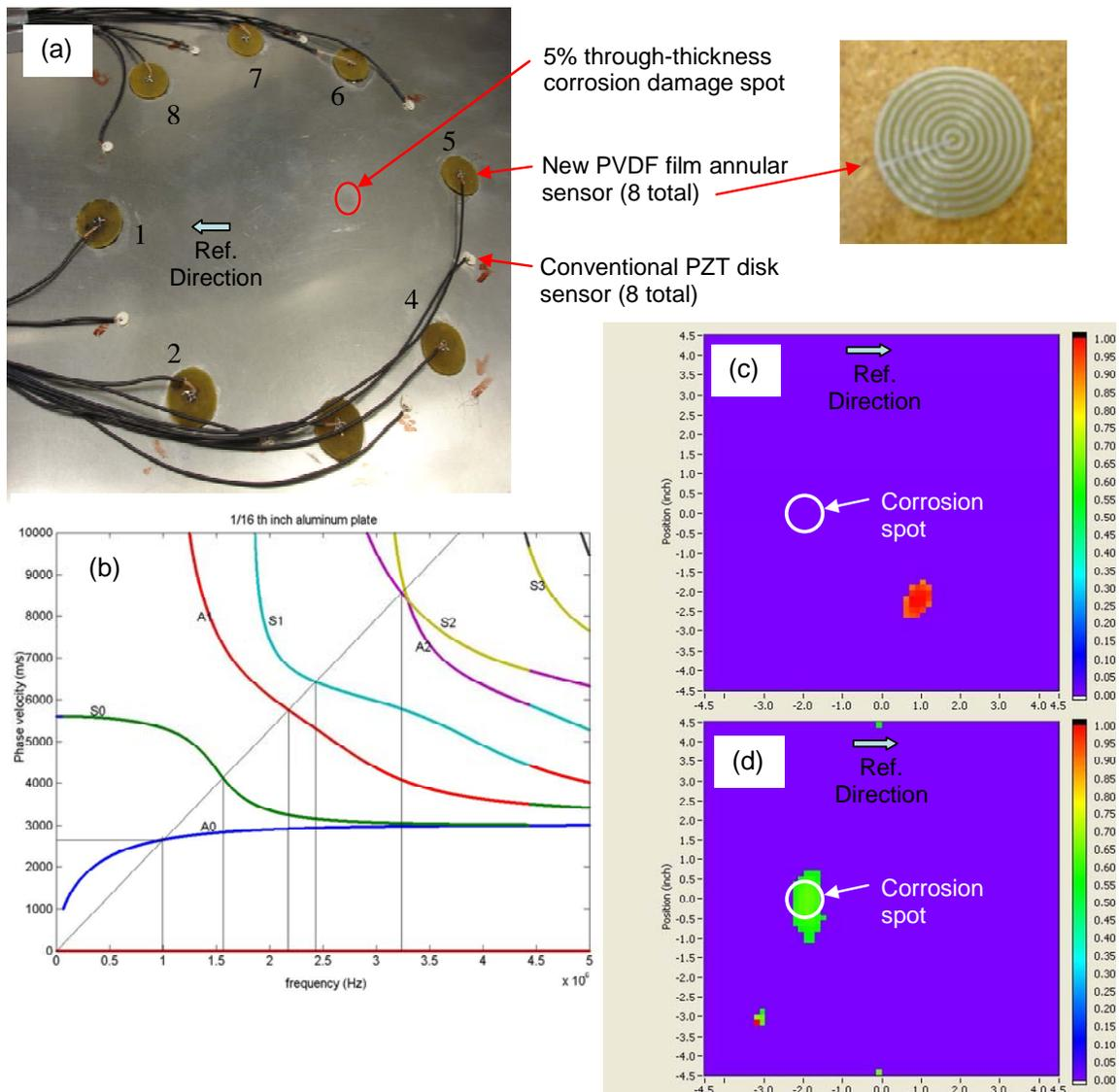
Figure 5: Corrosion damage detection, (a) sensor arrays enclosing the damage, (b) dispersion curves for aluminum plate with annular array activation line shown, (c) tomogram from PZT sensors did not identify defect and show a false positive, (d) tomogram from PVDF sensors identified corrosion in the presence of surface water.
