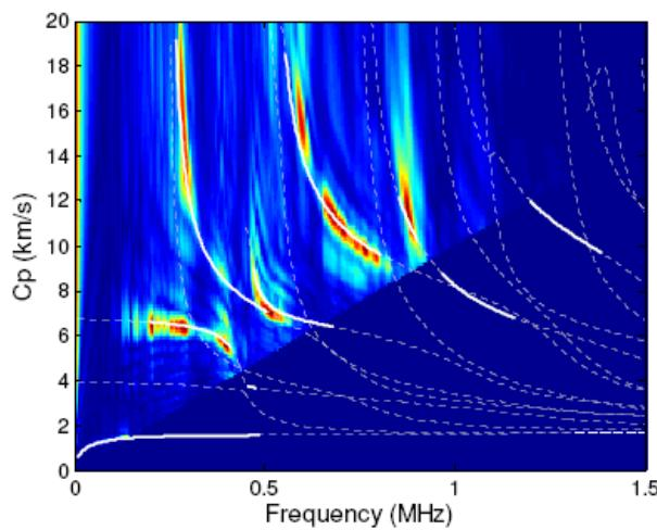
**Figure 7: Experimentally determined dispersion regions overlaid upon dispersion curves with optimal regions based upon excitability, skew angle, and attenuation [Gao, 2007].**
