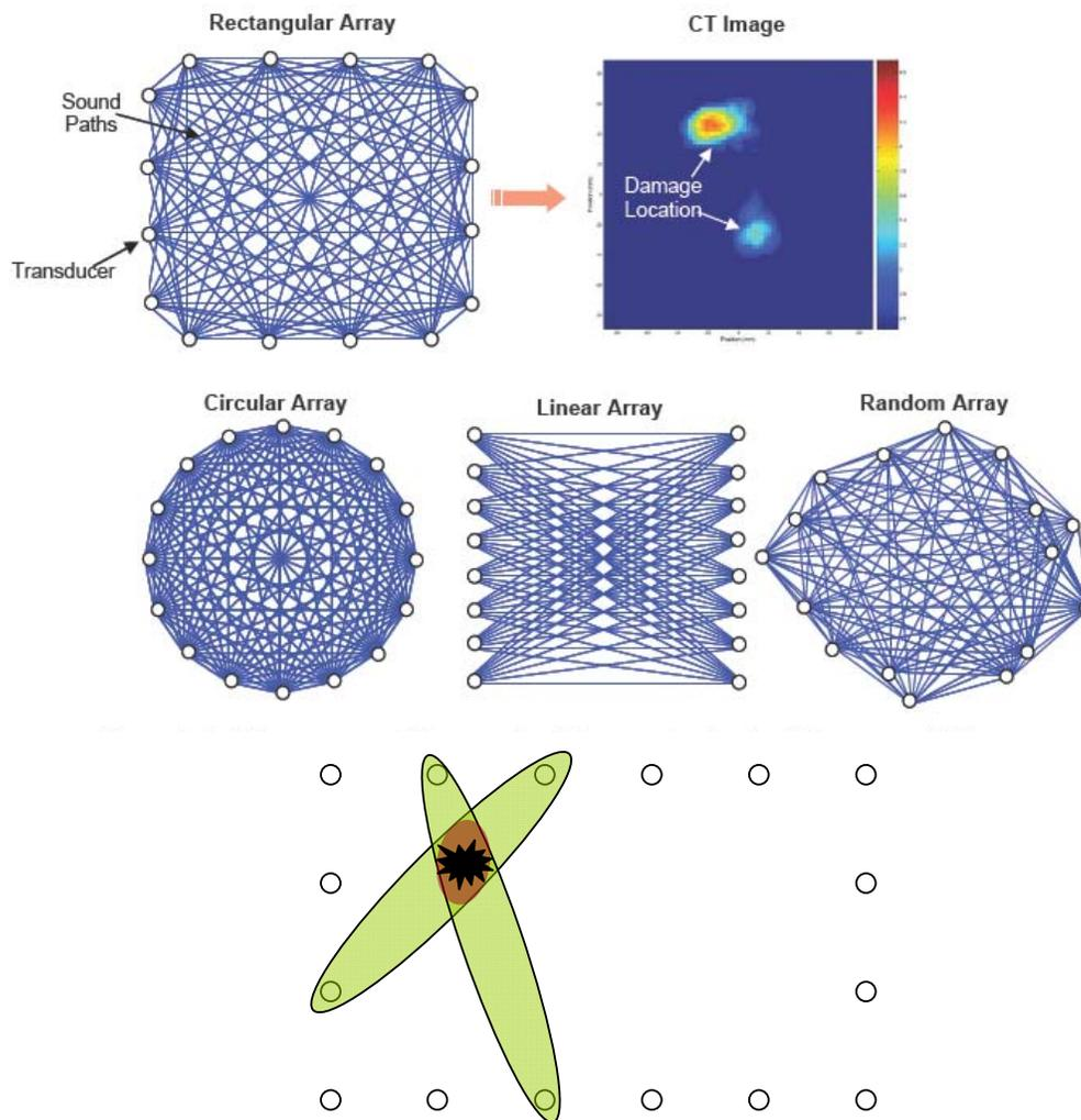
Figure 3: Schematic of sensor arrays showing chords between sensors and a computed tomographic image of damage.
