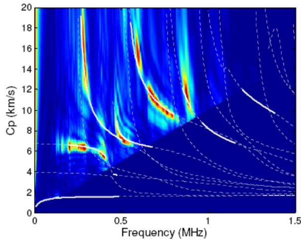
Figure 7: Experimentally determined dispersion regions overlaid upon dispersion curves with optimal regions based upon excitability, skew angle, and attenuation [Gao, 2007].
