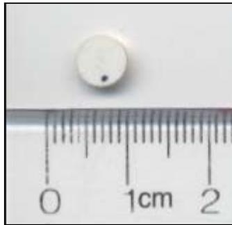
Figure 1: Surface mountable PZT sensor.
