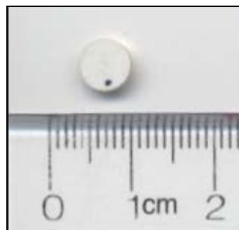
**Figure 1: Surface mountable PZT sensor.**
