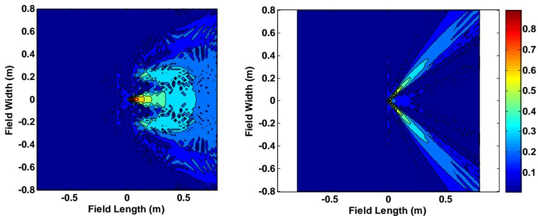
Figure 8: Beam forming at 45 degrees in a unidirectional composite plate with a nine element linear array of sensors using a delay-and-sum algorithm, (a) failed due to improper selection of mode and frequency, (b) successful due to understanding the underlying wave mechanics [Yan and Rose, 2007].
