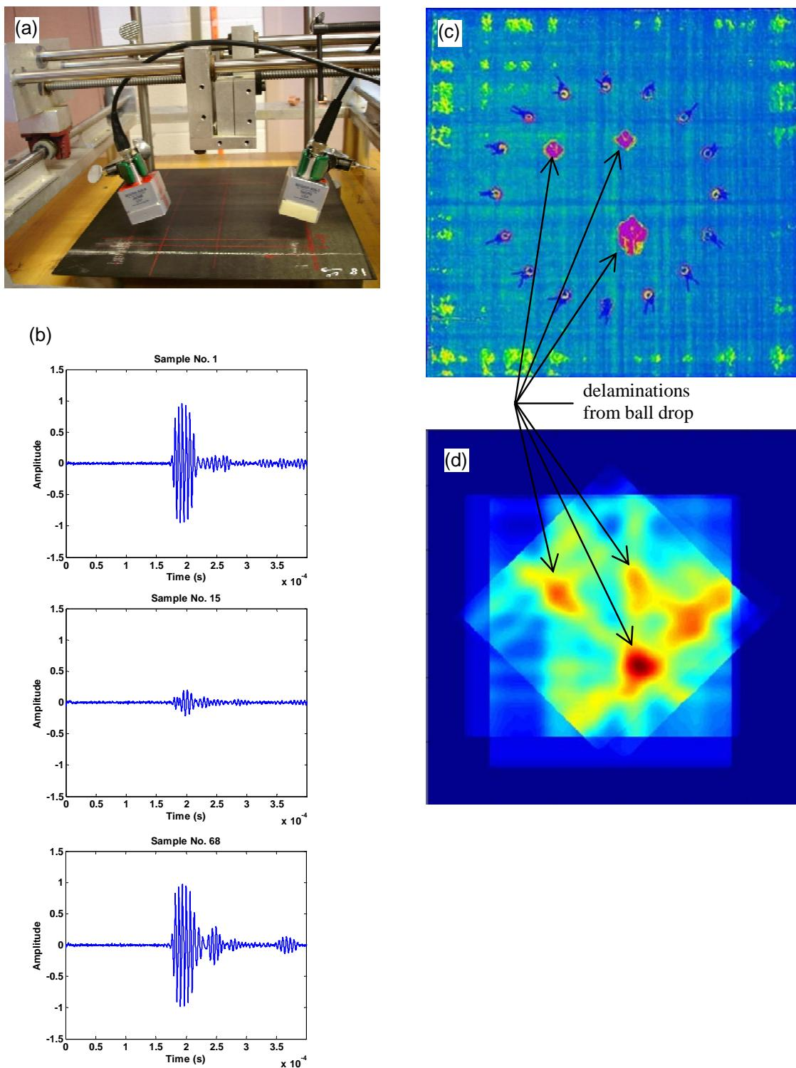
**Figure 4: Delamination detection with air coupled transducers and imaging; (a) air coupled transducers set off from composite plate, (b) sample signals received by air coupled transducer, (c) C-scan image, (d) air coupled transducer image.**
