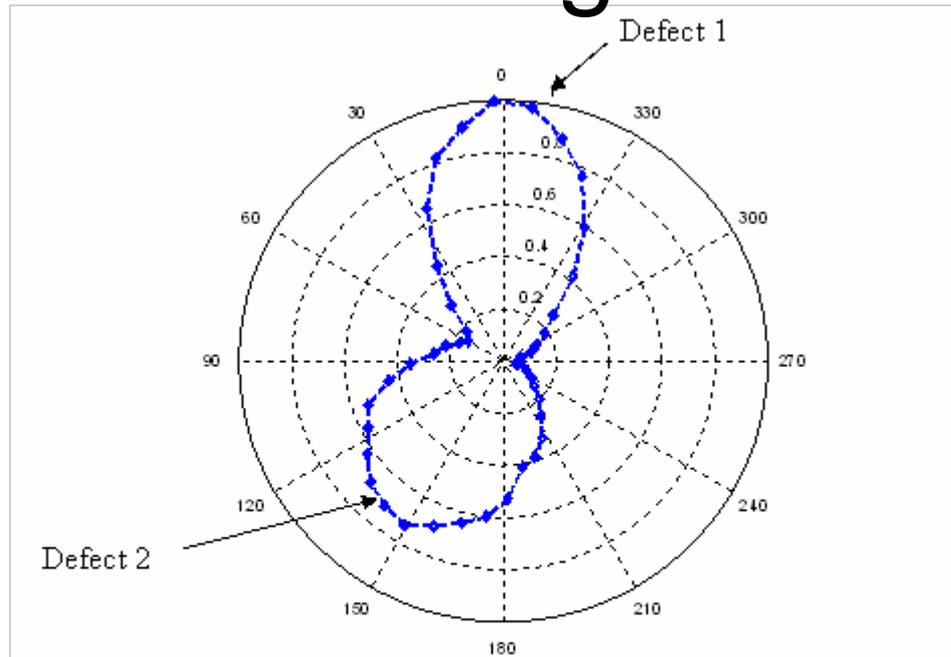
Figure 6. Maximum reflected echoes within the distance range: 12.5ft~20.8ft by applying 16-channel phased-array focusing. Circumferential length of each excitation channel is 22.5°. 35kHz T(0,1) wave group is focused at 15.4ft and 44 different circumferential locations.
