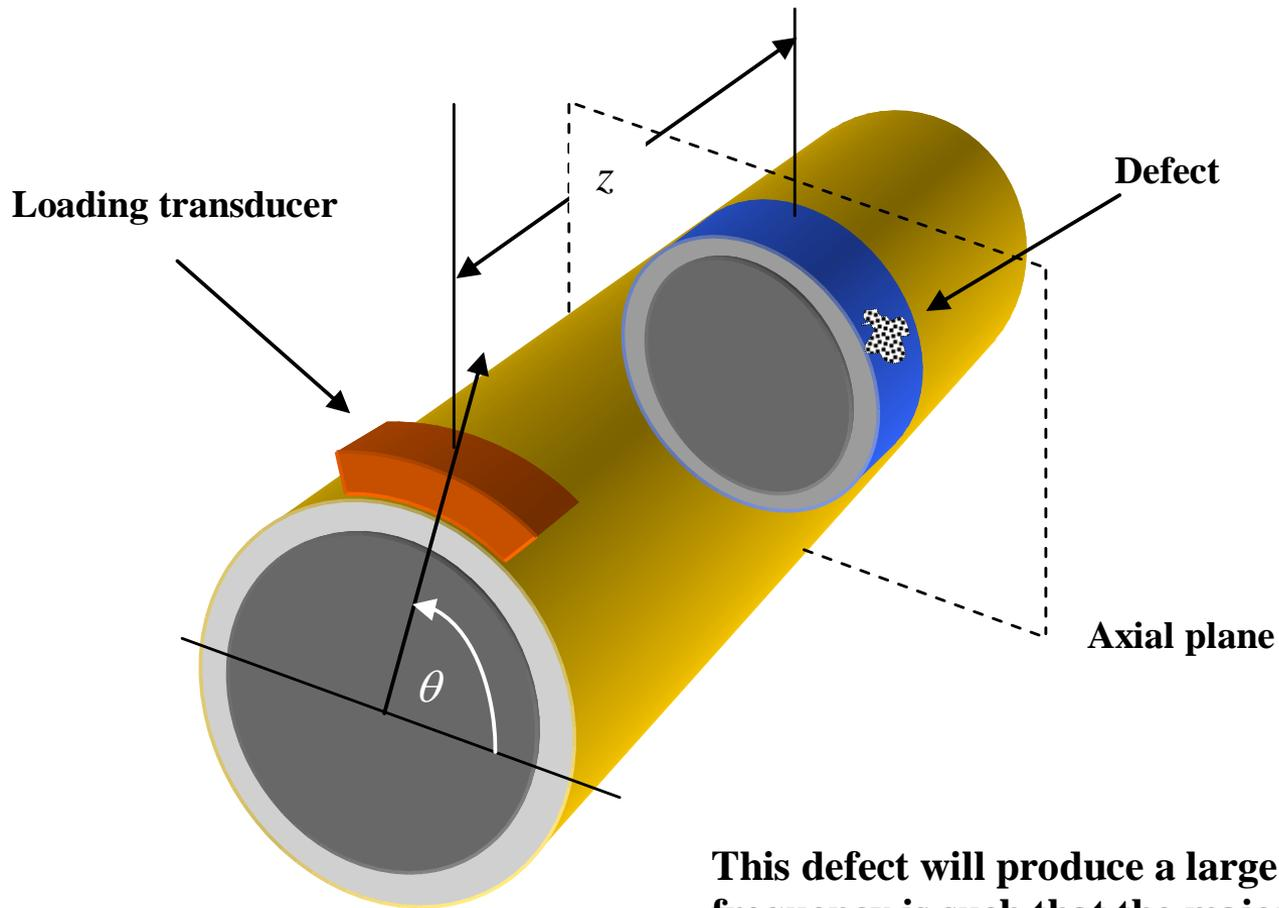
**This defect will produce a large response if the frequency is such that the major lobe of the displacement profile is located near or on it.**
