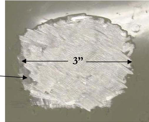
“Hidden” surface showing embedded sensor array
