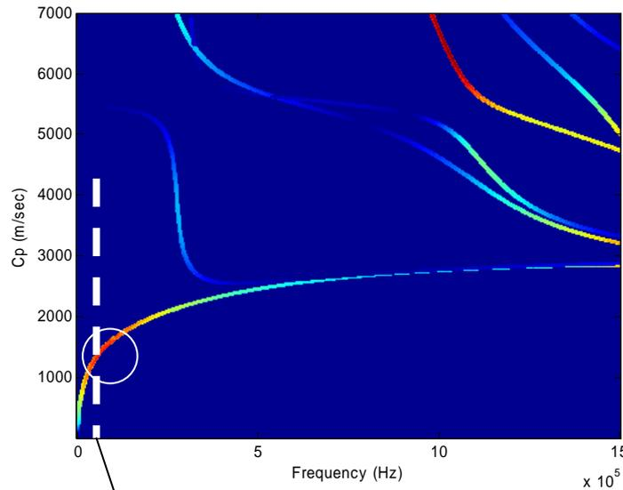
Use high energy transducer around 50 kHz to generate high interface shear stress, hence to de-ice.
