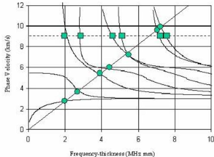
c). Mode excitation zones (Angle beam shoe—constant phase velocity [horizontal line] determined from Snell's Law for a given angle. Comb transducer excites modes with a constant wavelength [sloped line] determined by the spacing of the elements.)
