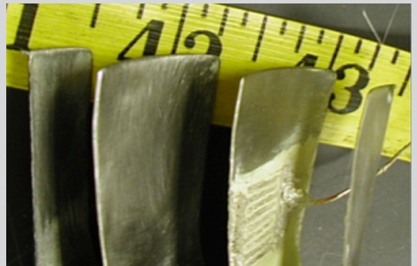
Figure 2. Functional spray-on bismuth titanate transducer on curved turbine blade fin
