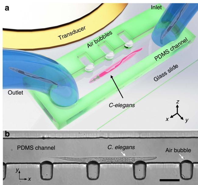
**Figure 1 | Design and operation of the acoustofluidic rotational manipulation (ARM) device.** (a) A schematic of the experimental setup. The piezoelectric transducer that generates acoustic waves is placed adjacent to the microfluidic channel. The acoustic waves actuate air microbubbles trapped within sidewall microcavities. (b) An optical image showing a mid-L4 stage *C. elegans* trapped by multiple oscillating microbubbles. Scale bar, 100  $\mu\text{m}$ .
