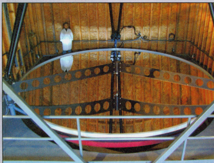
Figure 1. The University of British Columbia's Large Zenith Telescope has a 6-m aperture, making it the third-largest optical telescope in North America. The rotating liquid mirror, weighing approximately 3 tons, is the largest ever built. The rotational speed of the bowl containing the mercury controls the shape of the lens and can be controlled to within one part per million. Courtesy of Dr. Paul Hickson, University of British Columbia.
