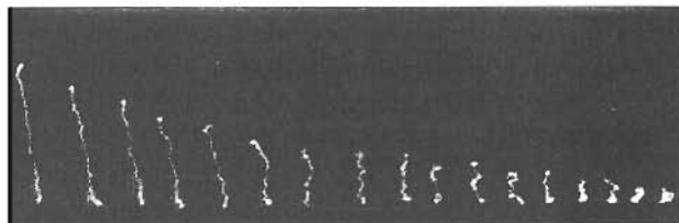
Fig. 4. Relaxation of a DNA molecule after hydrodynamic stretching is shown here in 2.5 second increments. Reprinted with permission from [16], P. K. Wong et al., J. Fluid. Mech. 497, 55 (2003). © 2003, Cambridge University Press.
