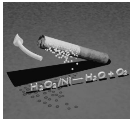
Figure 5. Illustration of rotary motion of a gold/nickel nanorod anchored via the gold end to a silicon surface and propelled into a circular orbit by oxygen nanobubbles evolved from the catalytic decomposition of hydrogen peroxide fuel to water and oxygen at the nickel end [23].
