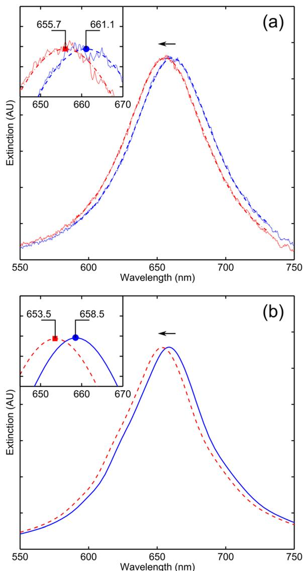
FIG. 2. (Color online) (a) Experimental extinction spectrum for gold nanodisk array. Raw data is shown as solid lines. The fitted curve for the initial position (dashed line) and the final position (dashed-dotted line) are shown as dashed lines. The insert displays a closer view of the peak positions. (b) The extinction spectra for the initial position (solid line) and the final position (dashed line) of the extinction spectrum simulated using DDA for the experimental conditions.
