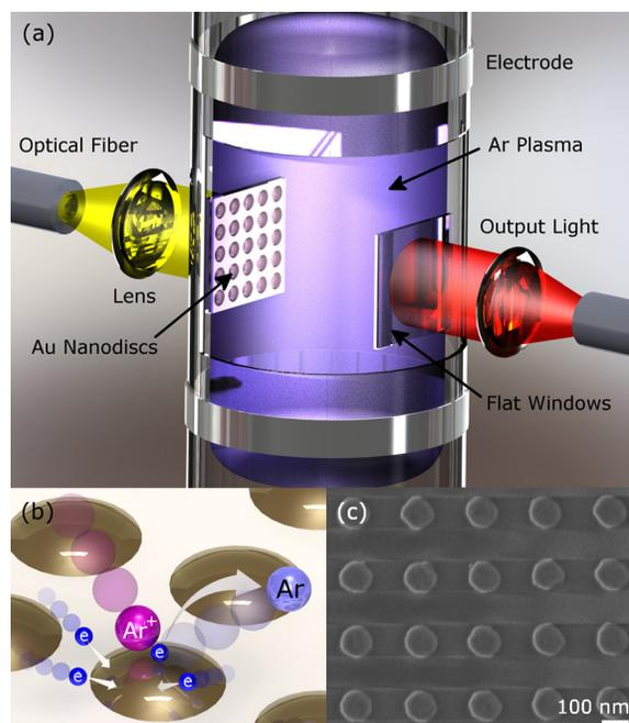
FIG. 1. (Color online) Experimental setup and device used in the experiment. (a) Schematic of the vacuum chamber, sample position, and optical setup. (b) Working mechanism for charging by plasma. (c) SEM image of the gold nanoparticles.
