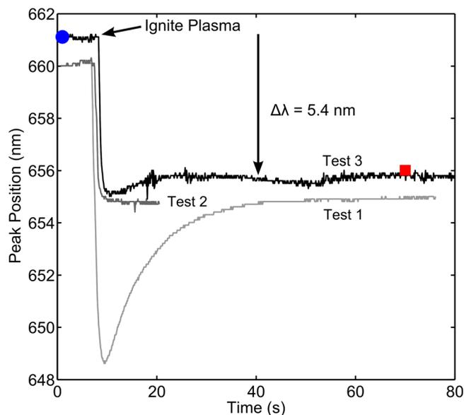
FIG. 3. (Color online) Dynamic response of the LSPR peak shift for three separate tests with a single nanodisk sample. The peak position of the fitted curve was recorded every 0.1 s. The blue circle and red square indicate the data points corresponding to the peak position of the initial and final curves plotted in Fig. 2(a), respectively.
