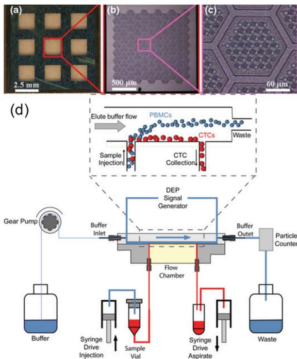
**Fig. 3** (a–c) Images of a 3-D microfilter, used for size-based mechanical separation of CTCs, at different magnifications. (d) Schematic of a dielectrophoretic CTC separation device, with detail provided for the flow chamber where an electrode sheet along the chamber floor generates an AC voltage to spatially separate CTCs from PBMCs via a DEP force. Reproduced from ref. 23, 27 with permission from AIP and Springer.
