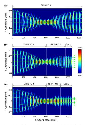
FIG. 3. FDTD-simulated acoustic wave propagation in (a) GRIN PC 1, (b) GRIN PC 1 + GRIN PC 2, and (c) GRIN PC 1 + GRIN PC 3 at the design frequency of 17.78 kHz ( $\Omega$ =0.25). The line-source-width is 400 mm wide and the wave aperture at the output is (a) maintained, (b) 210 mm, and (c) 140 mm.
