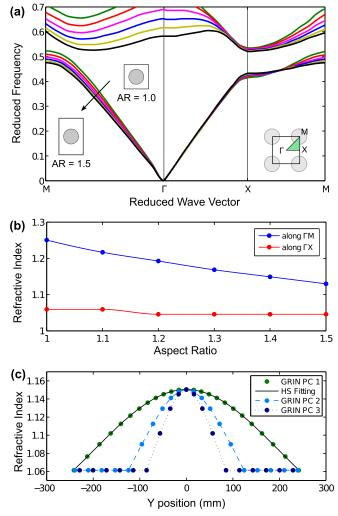
FIG. 2. (a) Band structures of rectangular-latticed steel/epoxy PC with different aspect ratios for the SV-mode BAW. (b) Refractive index of the steel/epoxy PC along  $\Gamma X$  and  $\Gamma M$  orientations against aspect ratio at reduced frequency of 0.25. (c) Effective refractive index profiles of three different GRIN PCs. Each can be fitted perfectly with a hyperbolic-secant function.
