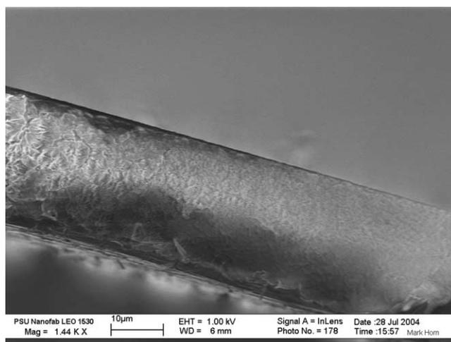
Fig. 2. Cross-section SEM micrograph of a parylene thin film grown normal to the nozzle assembly.
