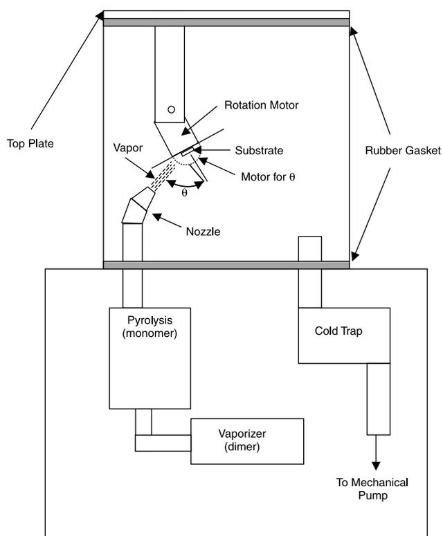
Fig. 1. Schematic of stepper motor and nozzle assembly used with the parylene deposition system. This system combines physical and chemical vapor deposition processes.
