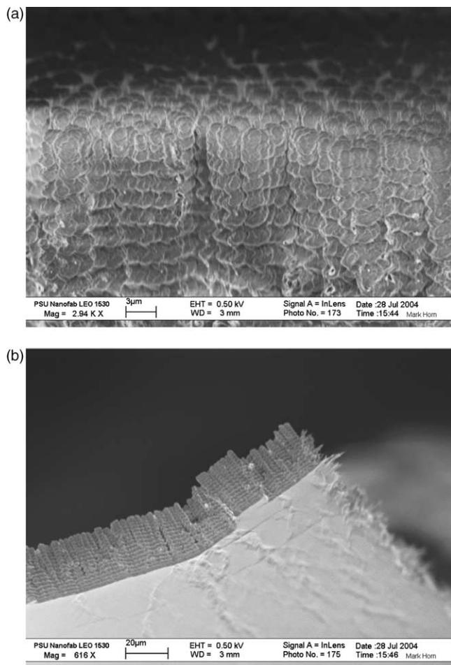
Fig. 3. SEM micrographs of a chiral sculptured thin film of parylene deposited at an angle  $\theta$  of  $80^\circ$  and a rotation speed of 0.025 rps (1.5 rpm). (a) 2.94K $\times$  magnification and (b) 616 $\times$  magnification.
