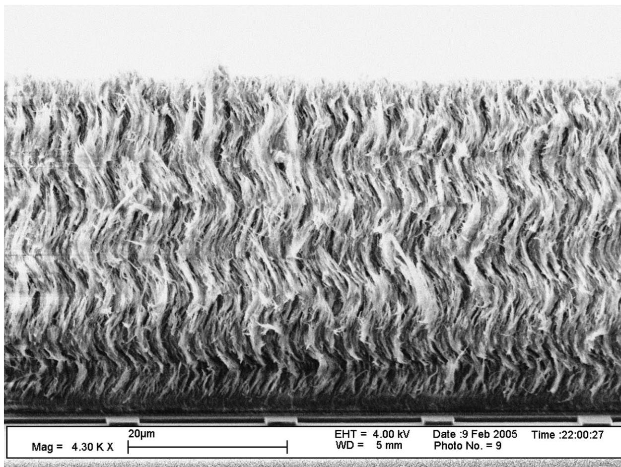
Fig. 5. SEM micrographs of a chiral sculptured thin film of parylene with small diameter size. The helical features are approximately 200 nm.
