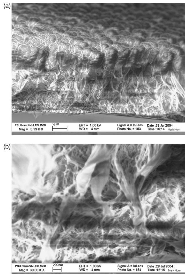
Fig. 4. Cross-section SEM micrographs of a parylene film deposited at an angle  $\theta$  of  $80^\circ$  and a rotational velocity of 0.167 rps (10 rpm). (a) 5.13 K $\times$  magnification and (b) 30 K $\times$  magnification. Note the fibrous nature of the film during initial growth (bottom) and the columnar structure near the top.
