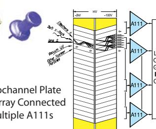
A Microchannel Plate (MCP) Array Connected to Multiple A111s
