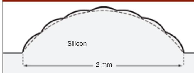
Cross section of the prismatic two-dimensional bioinspired texturing of the silicon surface.
