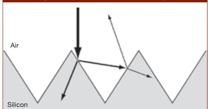
Transmission of light into silicon can be enhanced by texturing the exposed surface of silicon to trap the light rays by multiple reflections.
