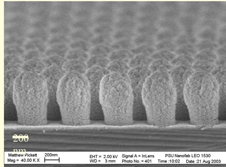
**SnO<sub>x</sub> STFs grown on photoresist patterns**
