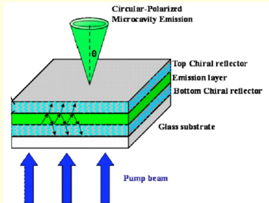
Fig. 3. Schematic of the light-emitting microcavity device incorporating two identical STF chiral reflectors sandwiching a layer of ALq3 molecules. Here,  $\theta$  denotes the emission cone. The oblique arrows drawn inside the layers simply underscore the back and forth bouncing of photons.
