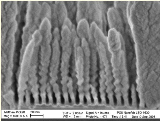
Single SiO<sub>x</sub> nanowire array grown on 60 nm e-beam resist
