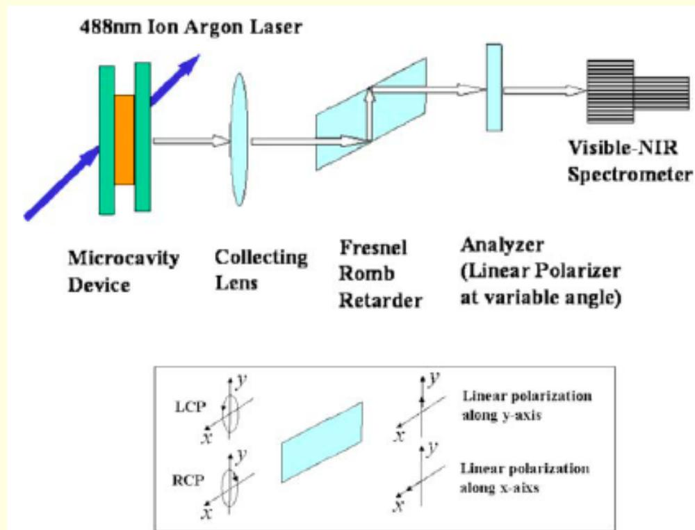
Fig. 4. Schematic of the optical bench used to characterize the circular polarization light-emitting device. The inset shows how a quarter-wave Fresnel-rhomb retarder converts LCP and RCP light beams to the linearly polarized light beams whose polarization directions are orthonormal.
