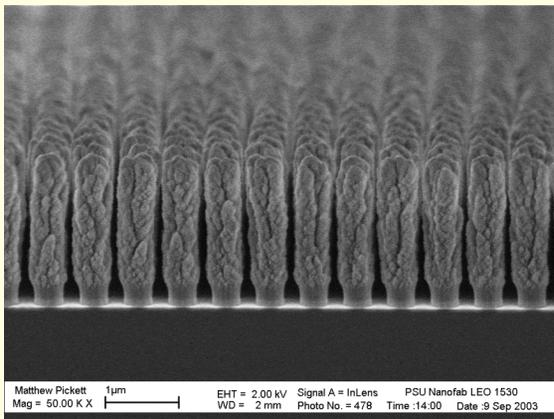
BCC array of SiO<sub>x</sub> nanocolumns
