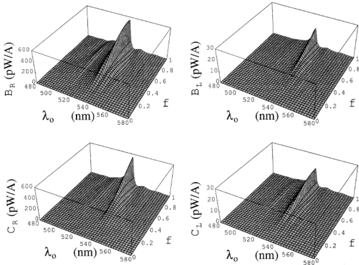
Fig. 1. Computed spectrums of the emission efficiencies  $\mathcal{B}_{R,L}$  and  $\mathcal{C}_{R,L}$  as functions of the fraction  $f$  of a chiral STF occupied by co-wound photon source filaments and the free-space wavelength  $\lambda_0$ . See the text for the constitutive and other parameters used. The Bragg regime for the selected parameters is  $\lambda_0 \in [513.4, 531.8]$  nm.
