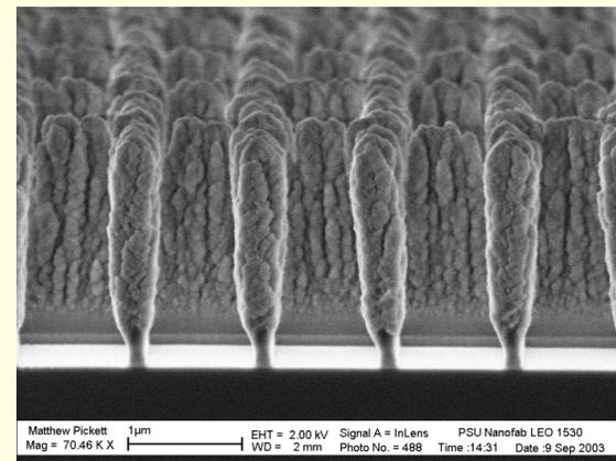
1µm x 1µm mesh of SiO<sub>x</sub> nanolines
