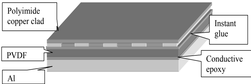
FIGURE 6. PVDF transducer element lay-up.
