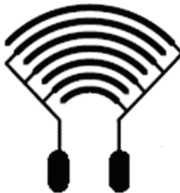
FIGURE 7. Annular array and section annular array with 90° span.
