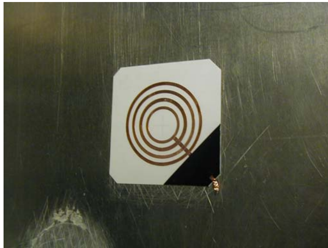
Figure 1. Lamb wave circular array.
